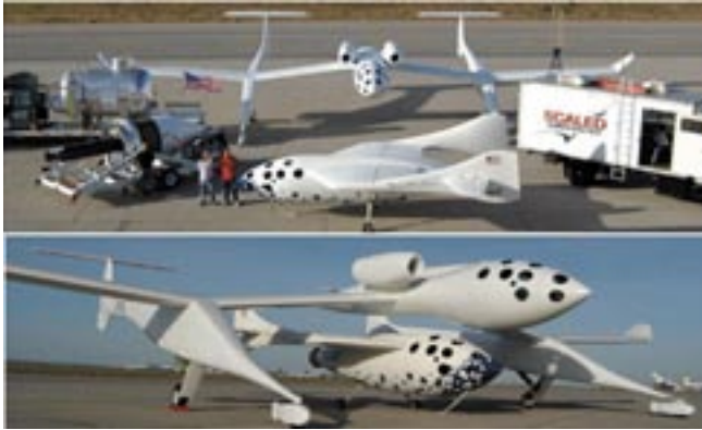
Scaled Composites' SpaceShipOne (foreground, top picture) and its drop-ship the White Knight (background, top picture). The bottom image shows SpaceShipOne and the White Knight together. CREDIT: Scaled Composites
